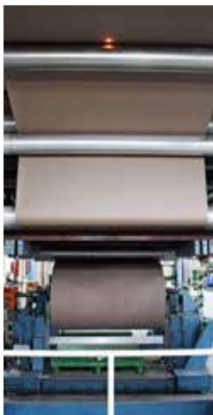
Finishing of the backing materials
