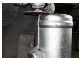
Grinding of cast parts
